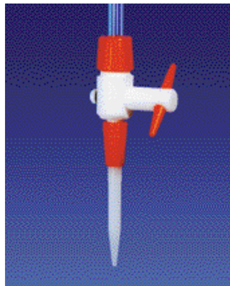
BURET STOPCOCK Supplied with 8mm diameter sidearm in borosilicate-B, or soda glass-S. Use suffix-B or -S in the reference number to indicate type. Bore is 2mm. Push-lock tip is polypropylene or glass.
